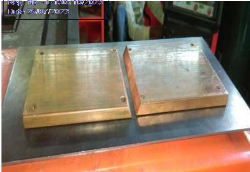
Fig: Fixture for weld plates
